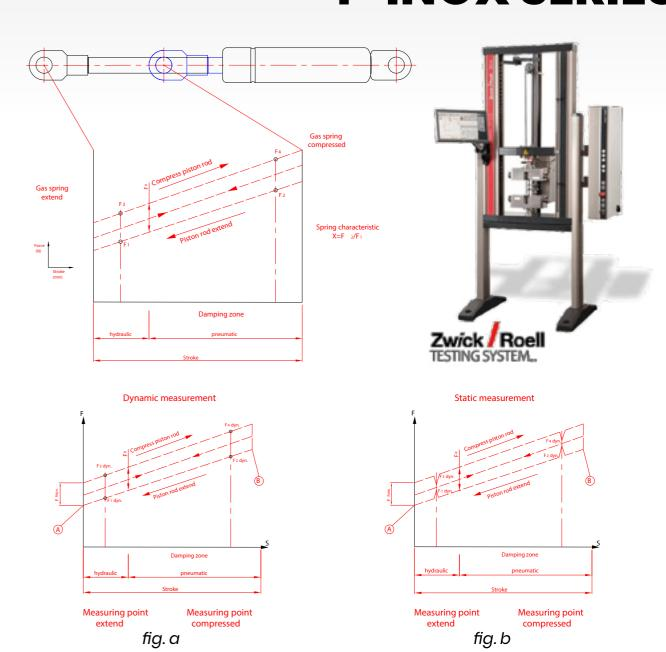
The spring characteristic curve shows the force path of the gas spring over the stroke, from the extended to the retracted state and back. The spring characteristic illustrates the balance of power of F2/F1. For the design of gas springs, the force FI is,in addition to the dimensions, the most important criterion. The force FI is measured 5mm before the end of the extension movement and thus defies the value of the spring force.
