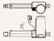
R = Extension cable, preset on motor cover (cable legth 50mm)
