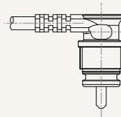
C = Y cable (direct cut, water proof, anti-pull)
