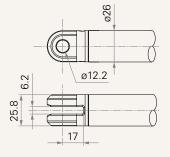
9 = Aluminum casting, U clevis, width 6.2, depth 17.0, hole 10.2, T bush
