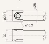
2 = Punched hole on inner Aluminum tube + plastic cap, without slot, hole 12.2, plastic bush
