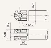
5 = Punched hole on inner Aluminum tube, wihout slot, hole 10.2, plastic bush
