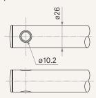
6 = Punched hole on inner Aluminum tube, wihout slot, hole 12.2, plastic bush
