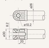
4 = Plastic, U clevis, width 8.2, depth 20.0, hole 12.2 (for push < 4000N, pull < 2500N)
