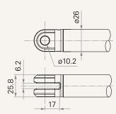
8 = Aluminum casting, U clevis, width 6.2, depth 17.0, hole 12.2
