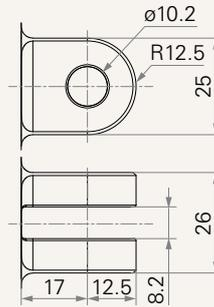
5 = Aluminum casting, U clevis, width 8.2, depth 17.0, hole 12.2
