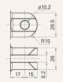
3 = Plastic, U clevis, width 8.2, depth 17.0, hole 12.2 (for push < 8000N)
