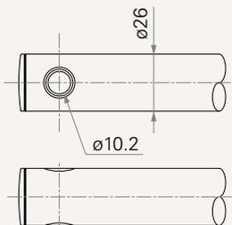
6 = Punched hole on inner Aluminum tube, without slot, hole 12.2, plastic bush
