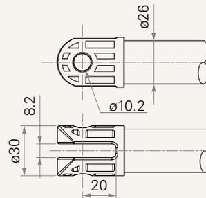
4 = Plastic, U clevis, width 8.2, depth 20.0, hole 12.2 (for push < 4000N, pull < 2500N)
